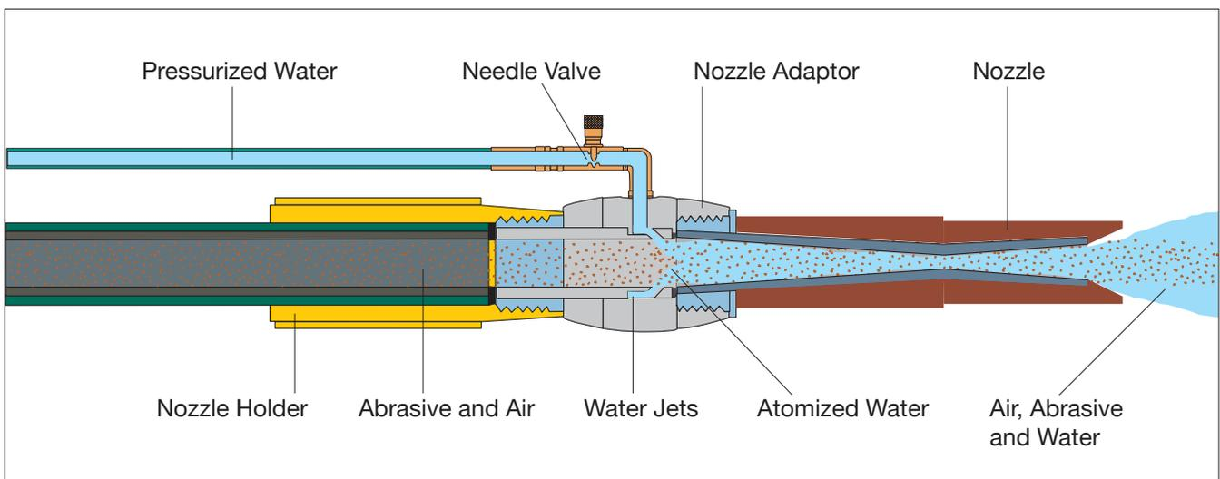
The Wetblast Injector is an economical kit that adds wet-blasting capability to most conventional dry-blast machines.
